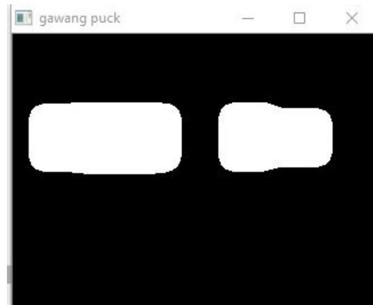
**Gambar 4.55** Hasil Proses *Thresholding* Warna Gawang Lawan
