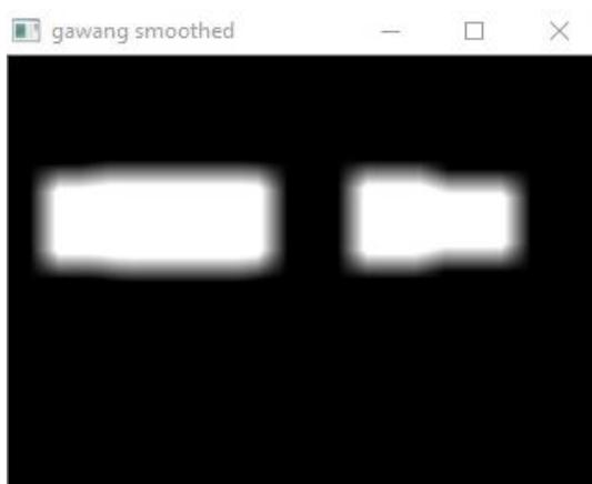
**Gambar 4.54** Hasil Proses 2D *Convolution* Warna Gawang Lawan
