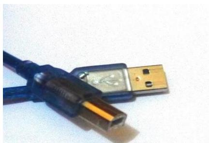
**Gambar 2.18** USB *Type* A to *Type* B
