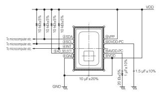
This circuit is an example to drive infrared array sensor "Grid-EYE", so that we will not take any responsibility of loss which is due to this circuit.
