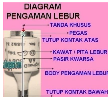
Gambar2.8 pengaman lebur ( fuse ) (Sumber: https://dunia-listrik.blogspot.com )
