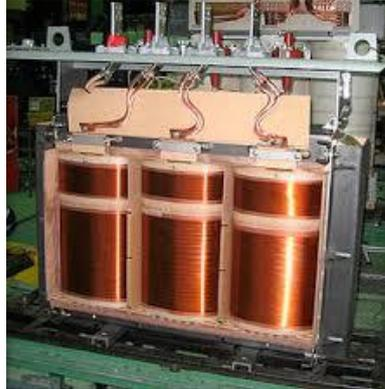
Gambar 2.5 Kumparan Transformator
