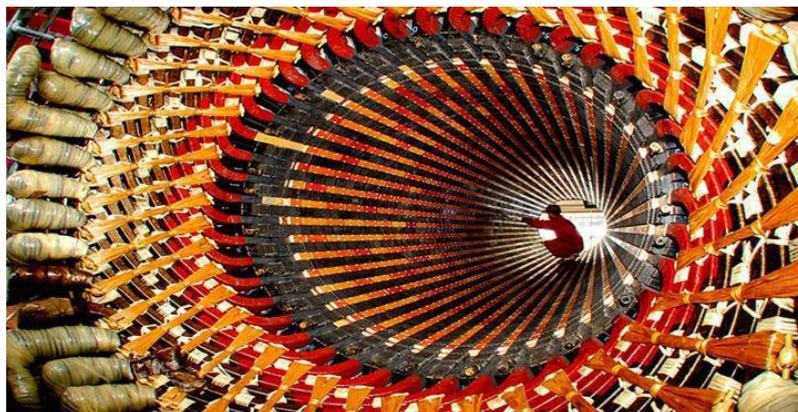
**Gambar 2. 2 Satator Generator Sinkron**
