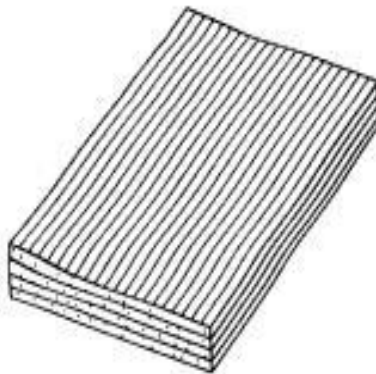
Gambar 2.2 Continuous Fiber Composite (Gibson, 2012).
