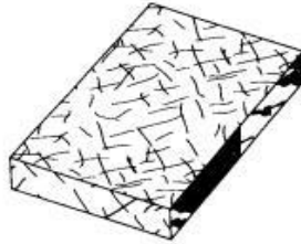
Gambar 2.1 Discontinuous Fiber Composite (Gibson, 2012).
