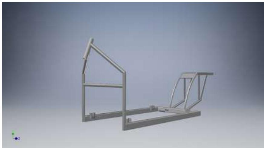
**Gambar 4.2** Rangka utama sepeda *treadmill hybrid helicle*
