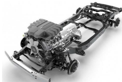
Gambar 2.8. Chassis terpisah ( http://www.toyota.astra.co.id )
