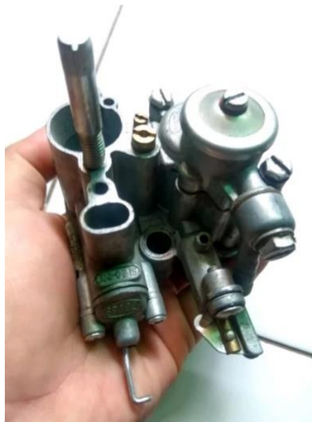
Gambar 3.2 Karburator vespa sprint spaco dellorto 20 20
