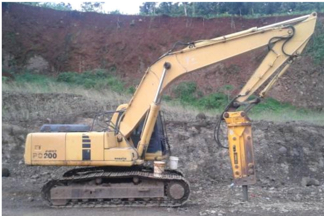
Gambar Excavator Breaker
