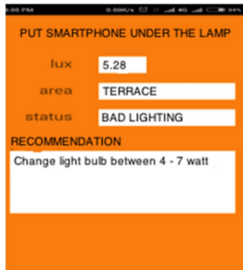
Fig. 7. Measurement for terrace, indicating bad lighting conditions, the software advice to change the correct light bulb.
