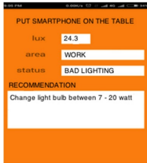
Fig. 6. Measurement for working area, indicating bad lighting conditions, the software advice to change the correct light bulb.
