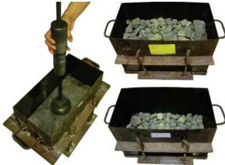
Gambar 3. 9 Pemadatan Benda Uji Perlapisan.
