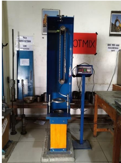
Gambar 3.10 Automatic Asphalt Compactor
