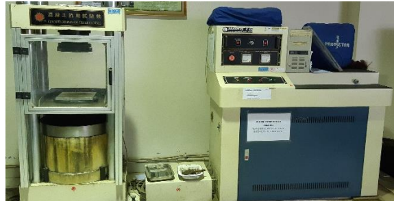
Gambar 3.15 Alat uji tekan Concrete Compression Tester Machine
