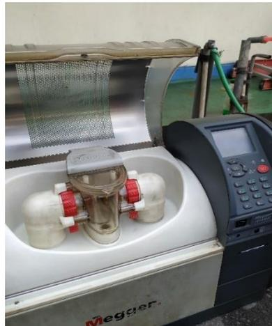
Gambar 4.7 *Laboratory Oil Dielectric Strength Test Set* (Megger - OTS 100 AF)
