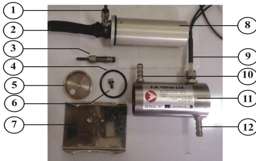
**Gambar 3.22.** Bagian-bagian *Heater*
