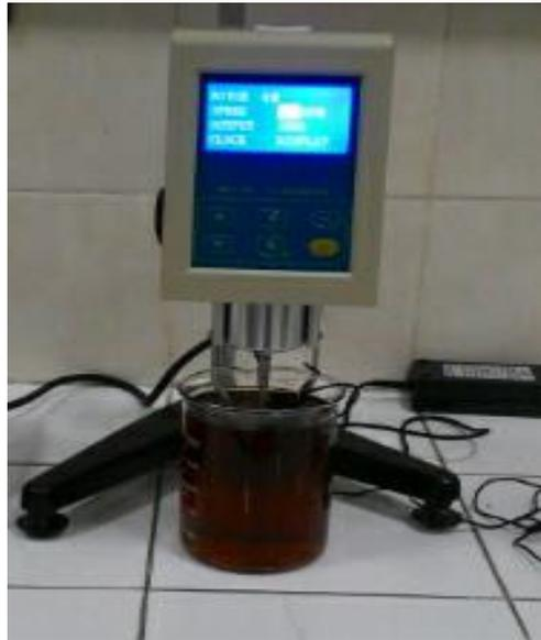
**Gambar 3.5.** Viskometer NDJ 8S
