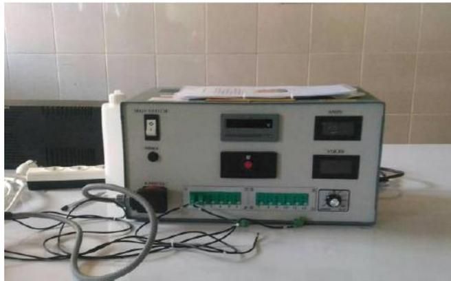
**Gambar 3.15.** *Thermal Conductivity of Liquid and Gases Unit*
