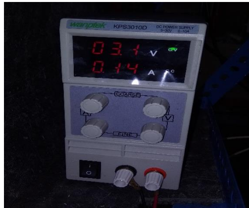
Gambar 3.5. DC Power Supply
