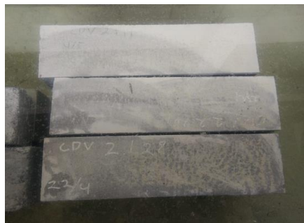
Gambar 3. 11 Proses perawatan benda uji ( curing )
