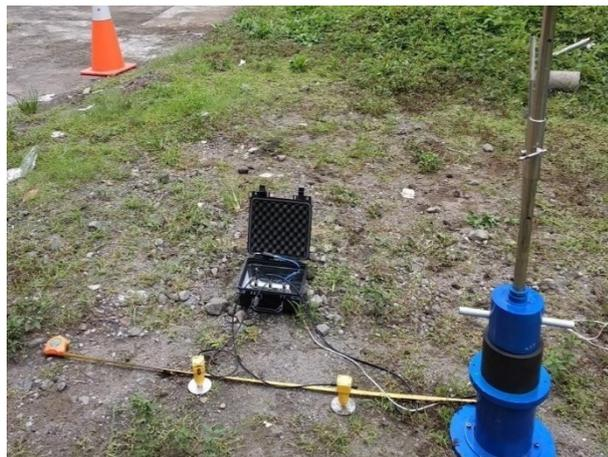
Gambar 3.4 Alat *Light Weight Deflectometer (LWD)*
