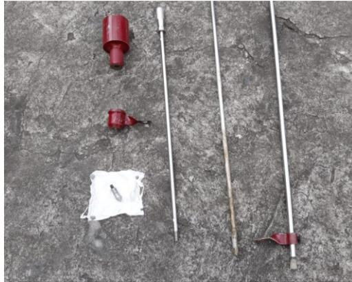
Gambar 3.5 Alat *Dynamic Cone Penetrometer (DCP)*
