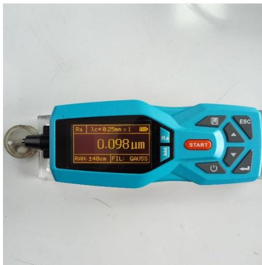
Gambar 3.3. *Surface Roughness Tester*
