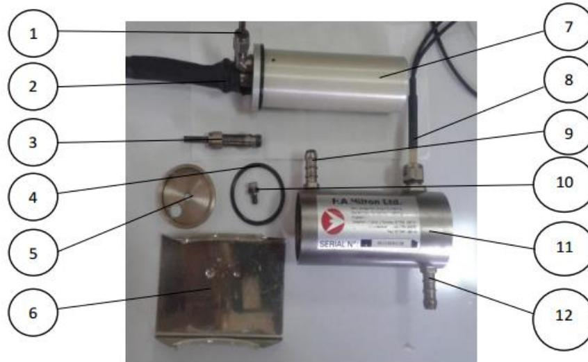
**Gambar 3.22** Bagian-bagian *heater*
