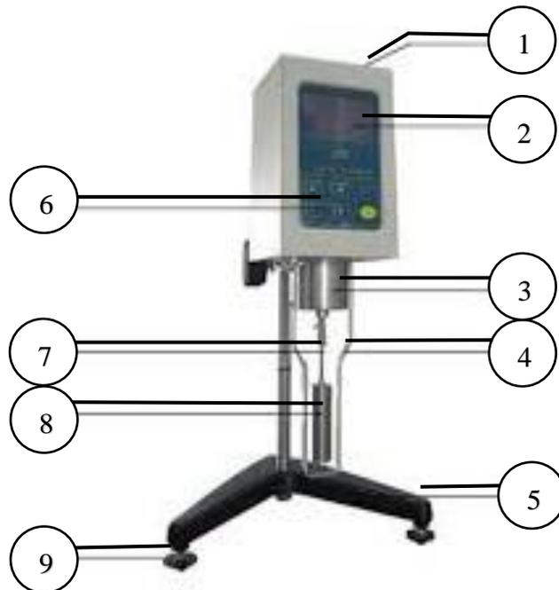
**Gambar 3.8.** Bagian-bagian viskometer NDJ 8S
