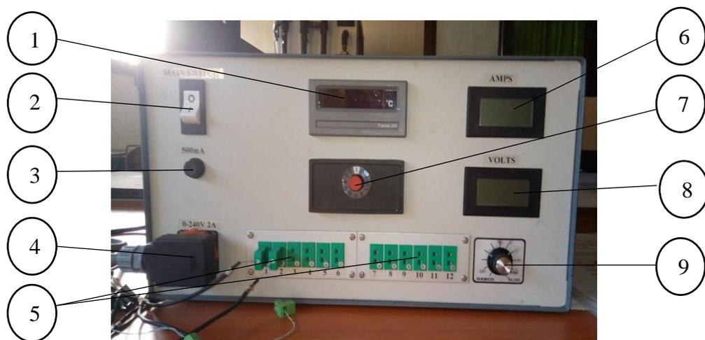
**Gambar 3.21** Bagian-bagian *heat transfer unit*
