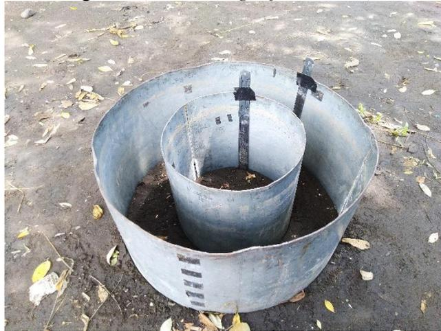
Gambar 1 Alat Infiltrometer cincin ganda (*double ring infiltrrometer*)
