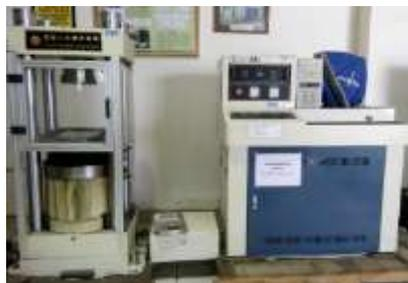
Gambar 3. 21 *Concrete compression tester machine*.
