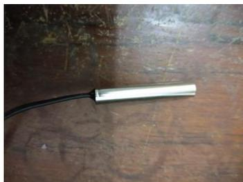
Gambar 2.6. Sensor NTC *Thermistor*
