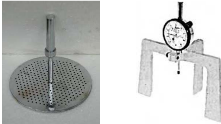
Gambar 4. 8 Pelat berlubang ( perforated plate ) dan tripod beserta arloji ukur
