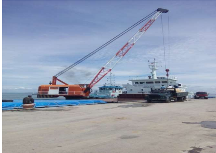
Gambar 4.12. Sistem Bongkar Muat Lift On-Lift Off (LOLO)
