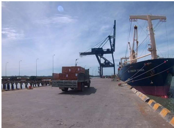
Gambar 4.11. Sistem Bongkar Muat Lift On-Lift Off (LOLO)
