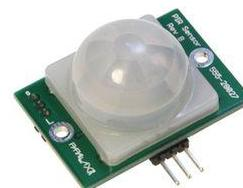
**Gambar 2.1** Sensor *PIR* (*Passive Infrared Receiver*)
