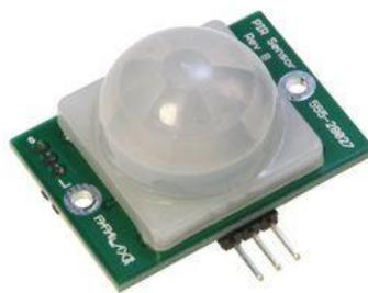
Gambar 2.1 Sensor *PIR* (*Passive Infrared Receiver*)
