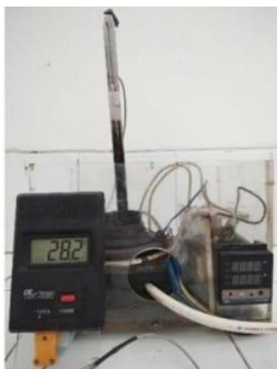
Gambar 3.9 Alat Uji *Flash Point*
