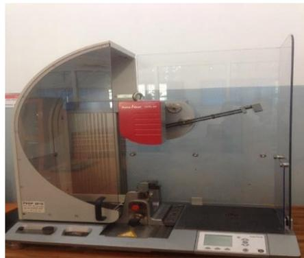
**Gambar 3.7.** Alat Uji Impak Charpy
