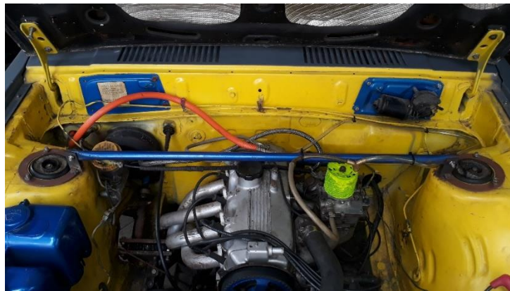
Gambar 4.11 Strut bar Development
