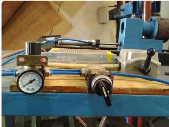
Gambar 4.19 Panel control friction welding
