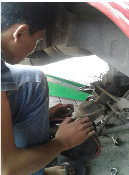
Gambar Proses penurunan unit Differential Mitsubishi Lancer SL
