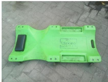
Gambar 3.9 *Mekanik Creeper*
