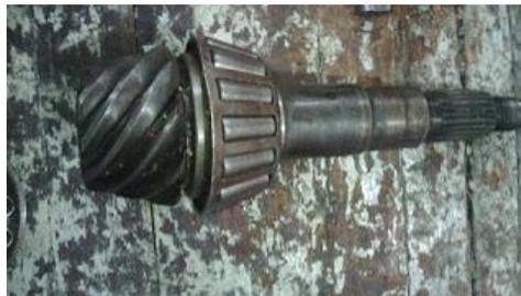
Gambar 2.14 *Drive pinion shaft*.
