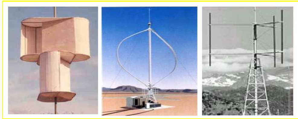
Gambar 2. 2 Turbin Angin Sumbu Vertikal (a) Savonius Rotor, (b) Darrieus Rotor, (c) H Rotor
