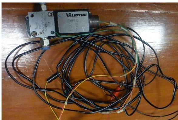
Gambar 3.17 *Pressure transducer*
