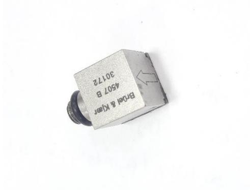
Gambar 3. 9 Accelerometer
