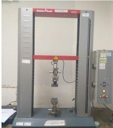
Gambar 3.13. Universal Testing Machine (UTM)
