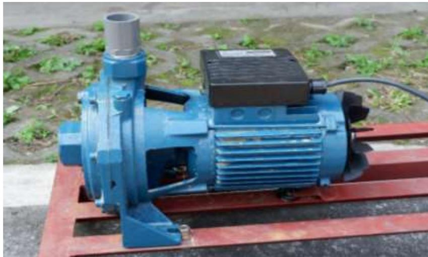
Gambar 3. 2 Pompa sentrifugal
