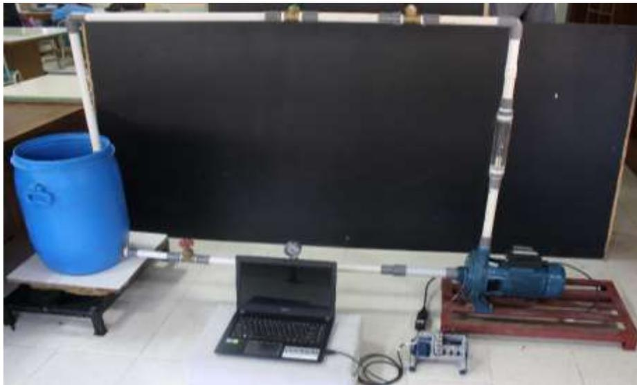
Gambar 3. 1 Rancangan Alat Test-Rig Kavitasi Pompa Sentrifugal
