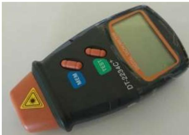
Gambar 3. 8 Tachometer digital
