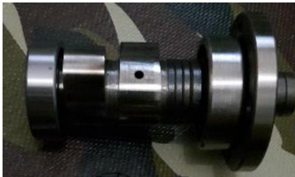
Gambar 2.12. Noken as (*Camshaft*)
