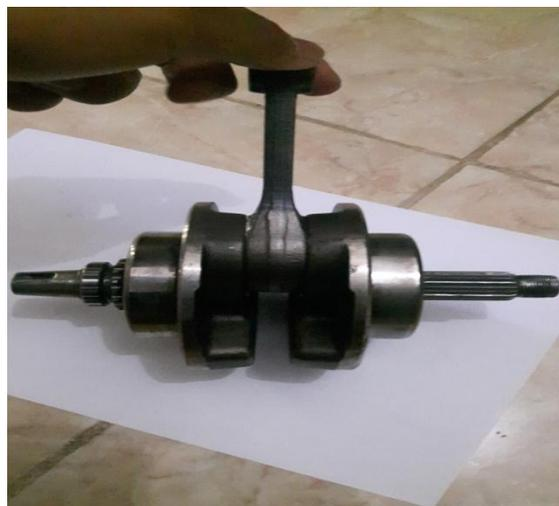
Gambar 2.8. Poros Engkol (*Crank shaft*)
