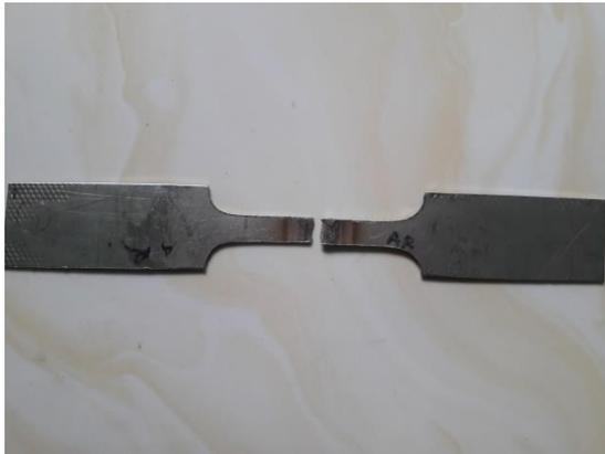
**Gambar 4.8** hasil patahan specimen 2 gas argon
