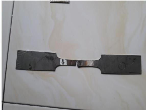
**Gambar 4.10** hasil patahan specimen 2 gas  $CO_2$
