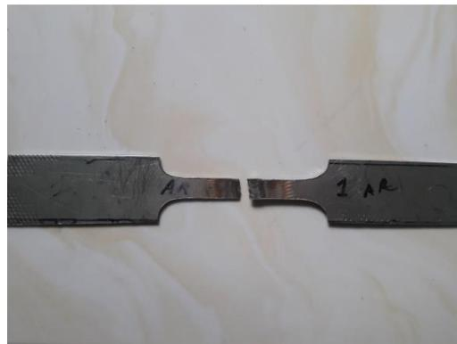
**Gambar 4.7** hasil patahan specimen 1 gas argon
