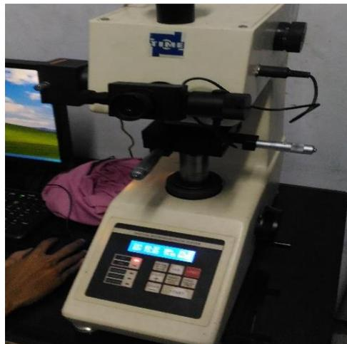
**Gambar 4.11** *Alat Microhardness Vicker Tester (Model 402 MVD S/N "V2D531")*.
