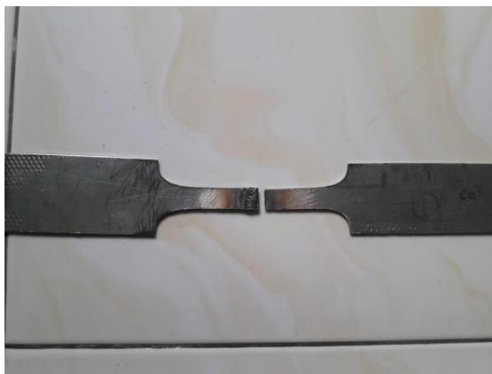
**Gambar 4.9** hasil patahan specimen 1 gas  $CO_2$
