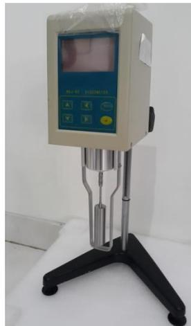
Gambar 3.11 Alat uji viskositas (*viscometer*)
