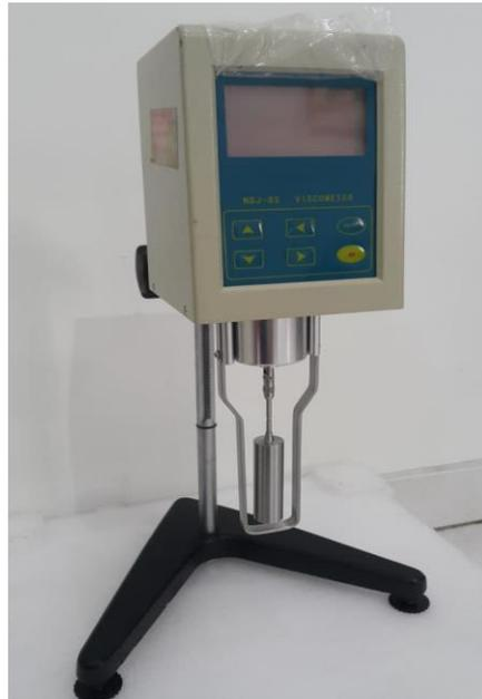
Gambar 3.11 Viskometer
