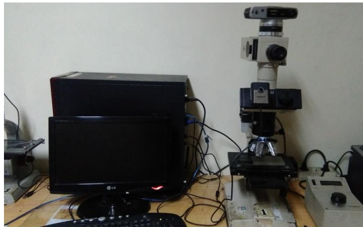
Gambar 3.5 Mikroskop optik ( Metallurgical Microscope Invertgo Tipe )
