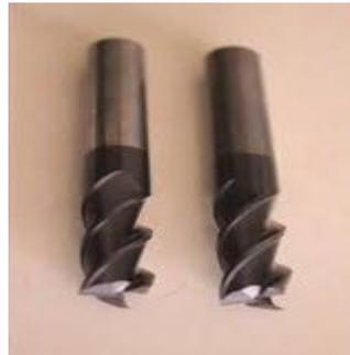
**Gambar 3.8.** Endmill 2 sphere diameter 6 mm
