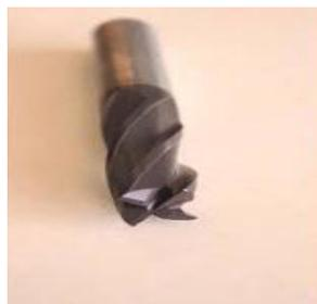
**Gambar 3.7.** Endmill 1 flat diameter 10 mm
