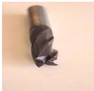
Gambar 3. 9. Endmill 1 flat diameter 10 mm
