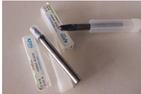
Gambar 3. 10. Ballnose diameter 6 mm
