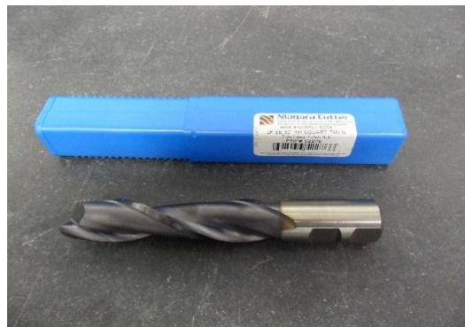
Gambar 3.5. Endmill 1 flat diameter 12 mm
