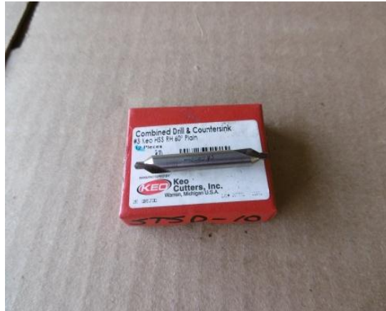
Gambar 3. 6 . Center drill diameter 10 mm
