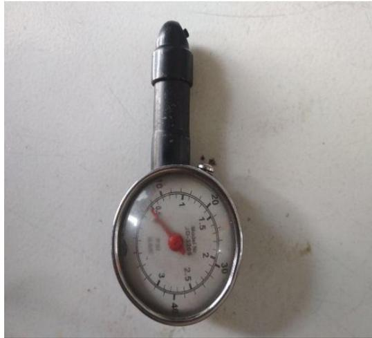
**Gambar 3.12.** *Tire Pressure Meter*
