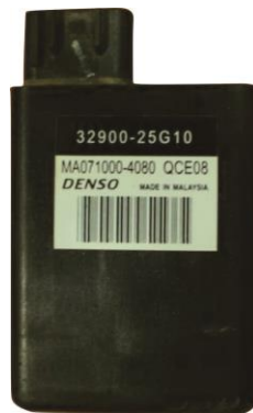
Gambar 3.2. CDI standar Suzuki Satria FU 150 cc
