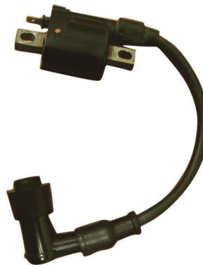
Gambar 3.4. Koil standar Suzuki Satria F 150 cc
